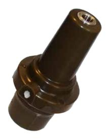
The connection of the HV-cables is made by cable bushings. The bushings are made of cast resin with moulded-in conductors. In addition, a screen is moulded in to control the electrical field and is also used as the main capacitor supplying the voltage indicating systems.
